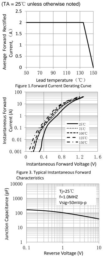
Figure 5. Typical Junction Capacitance
